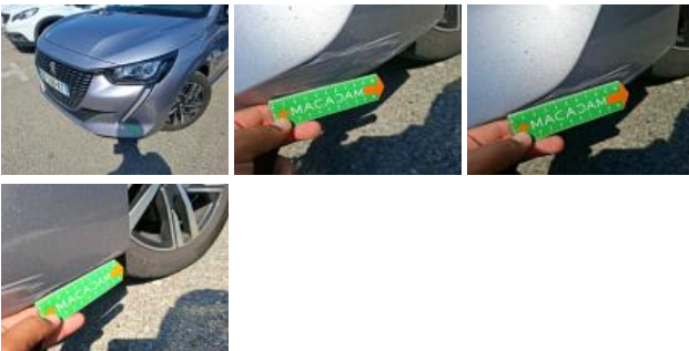
Door FR, Dent(s), Repair and paint (complete)
