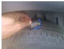
Tyre RL, Out of tolerance, Replace
