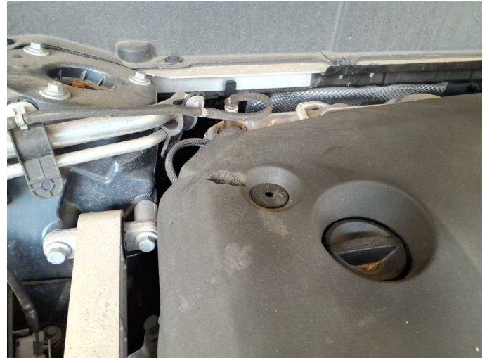
Damage 3: Engine: Engine cover - Damage caused by marten / rodent - Replace
