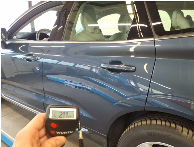
Repainting 2: Door - rear left side
