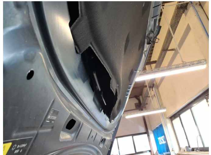
Damage 1: Bonnet: Insulation lining - Loose - Un- / install
