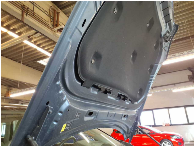
Damage 1: Bonnet: Insulation lining - Loose - Un- / install
