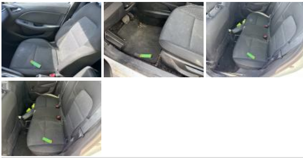
Headrest RR, Missing, Replace
