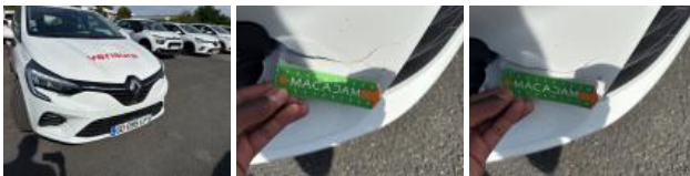
Bumper moulding FR, Broken, Replace
