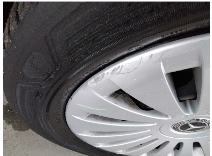
Damage 1: Wheel / tyres: Wheel cover - front right side - Scratch(es) - Replace
