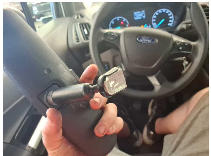
Damage 1: Instrument panel: Interior mirror - Loose - Un- / install
