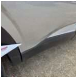
Damage Type small dents / small scratches
