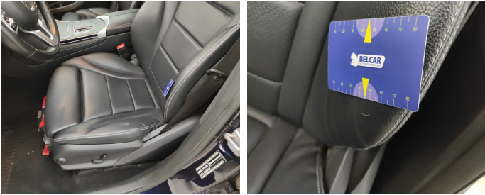
Seat Front Left / Bottom Coating / Replace-worn
