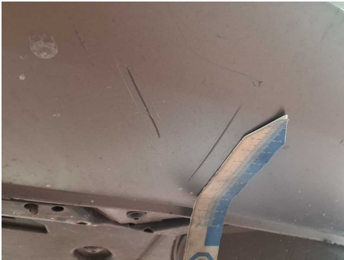
Damage 8: Front bumper: Spoiler (links + rechts + mitte) - Scratched - Loss in value
