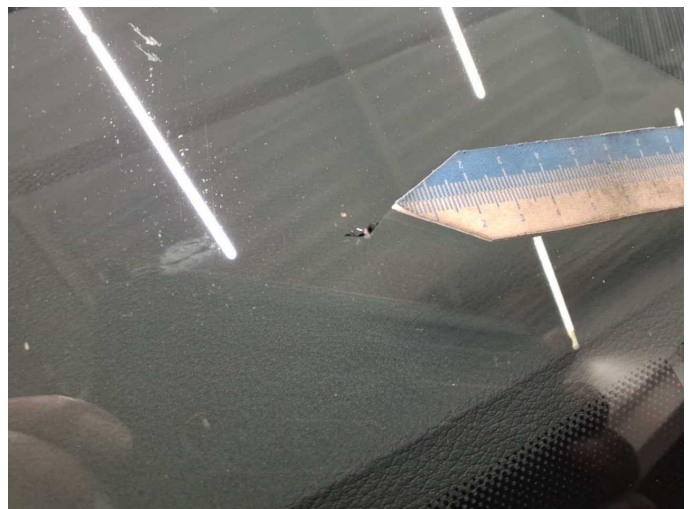
Damage 5: Vehicle glazing: Windscreen with lane departure assistant - Stone chips - Smart repair
