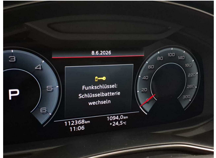
Damage 1: Equipment: Vehicle key with remote control (Batterie) - Due - Replace
