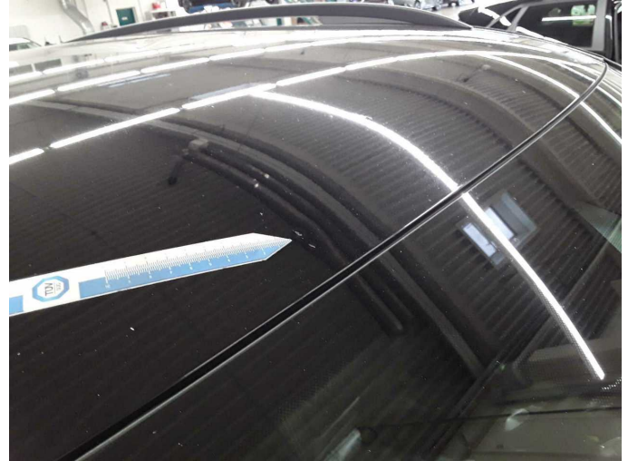
Damage 3: Roof: Roof - Dent / paintcoat damage - Smart repair
