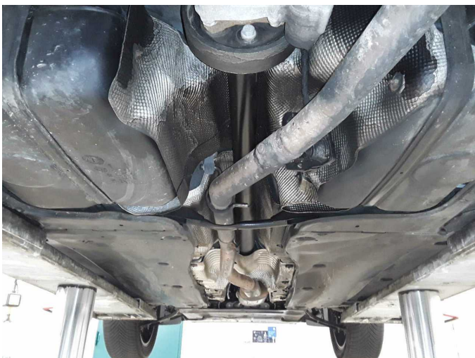
Damage 2: Body: Underbody (Ölspuren erkennbar) - Soiled - Perform diagnosis
