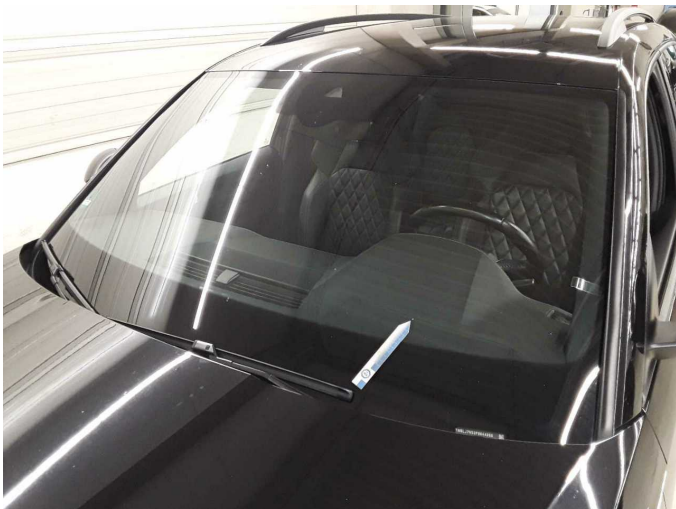
Damage 7: Vehicle glazing: Windscreen - Stone chips - Replace
