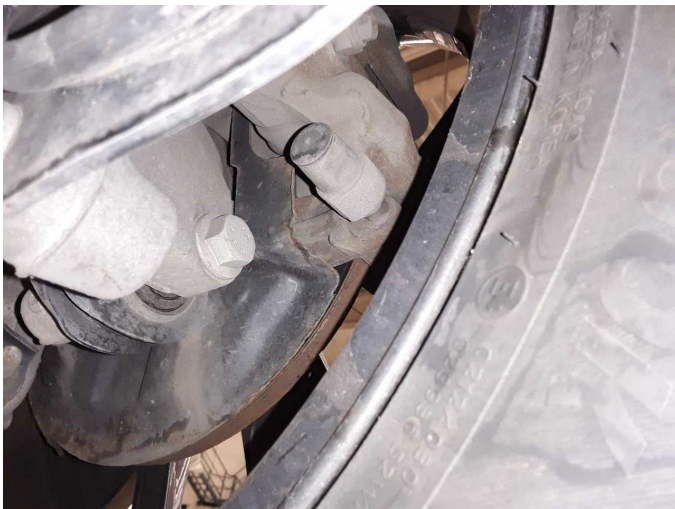
Damage 5: Braking system: Brake discs and pads - rear - Corrosion - Replace
