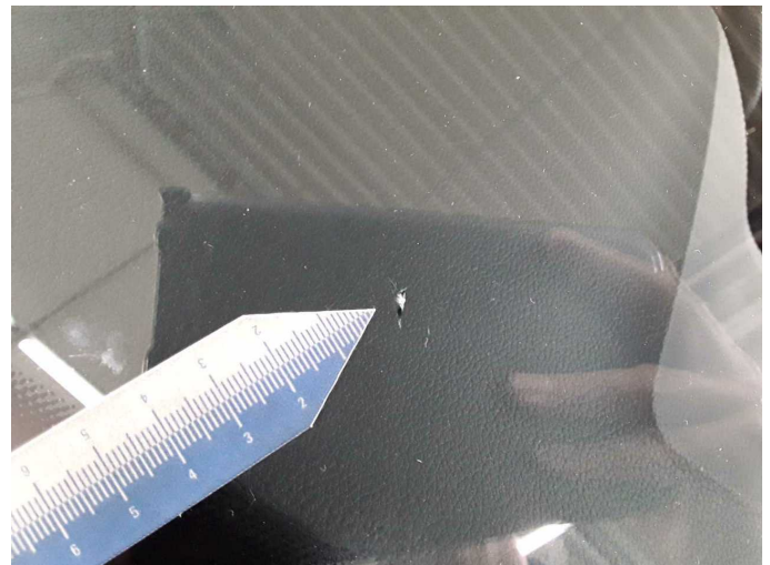
Damage 7: Vehicle glazing: Windscreen - Stone chips - Replace
