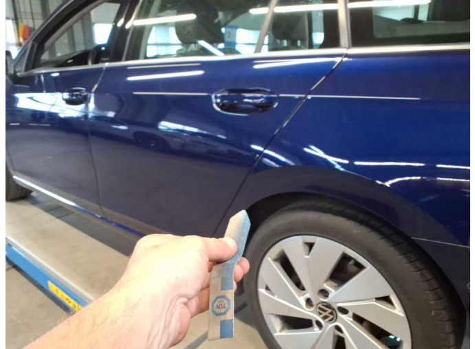
Damage 7: Side panel - rear left side: Side panel - Dent / paintcoat damage - Repair and paint
