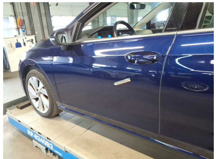
Damage 9: Door - front left side: Door - Dent / paintcoat damage - Repair and paint
