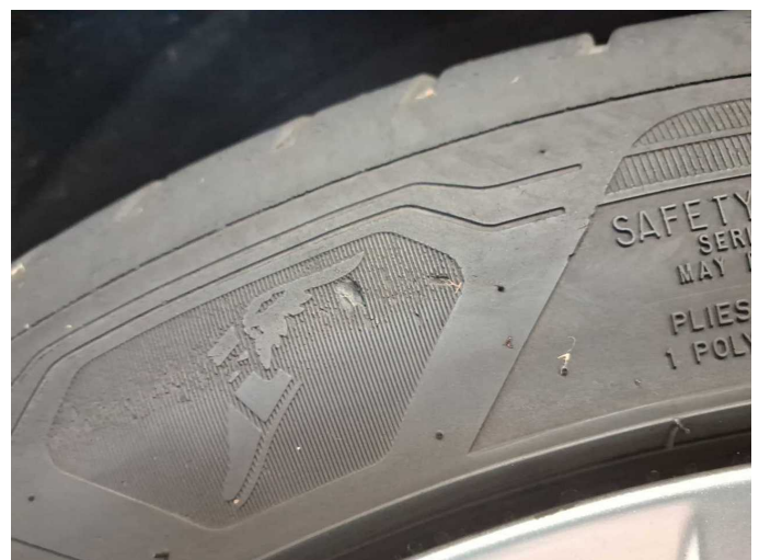
Damage 5: Wheel / tyres: Tyre - rear right side (Flanke) - Damaged - Replace
