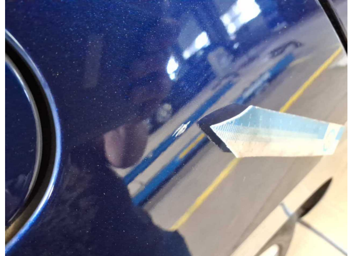
Damage 3: Side panel - rear right side: Side panel - Scratch(es) - Smart repair
