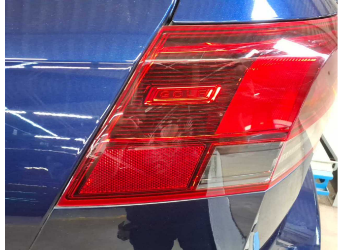
Damage 6: Tail light: Tail lamp - left side - Scratched - Replace
