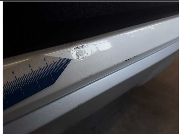
Damage #7: Rear bumper: Spoiler - Scratched - Replace
