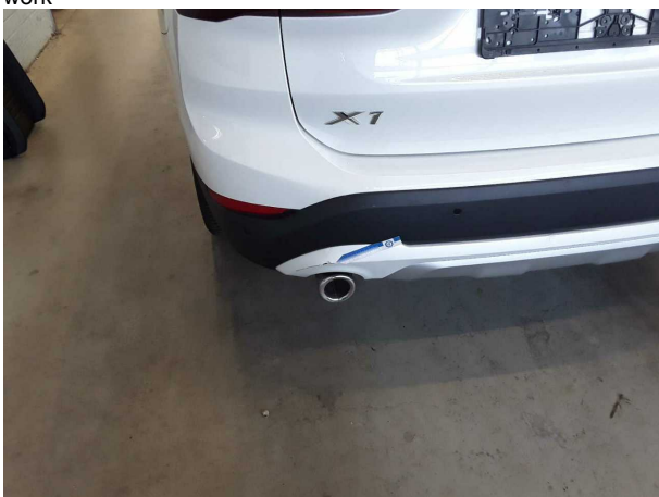
Damage #7: Rear bumper: Spoiler - Scratched - Replace
