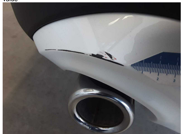
Damage #7: Rear bumper: Spoiler - Scratched - Replace
