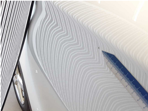
Damage #5: Door - rear right side: Door - dent(s) - Smooth repair work
