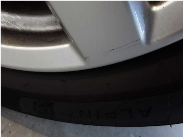
Damage #1: Wheel / tyres: Alloy rim - rear left side - Scratch(es) - No deduction
