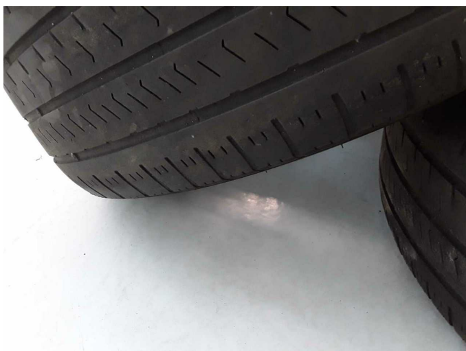
Damage 6: 2nd wheel set: 2 tyres - Worn - Replace
