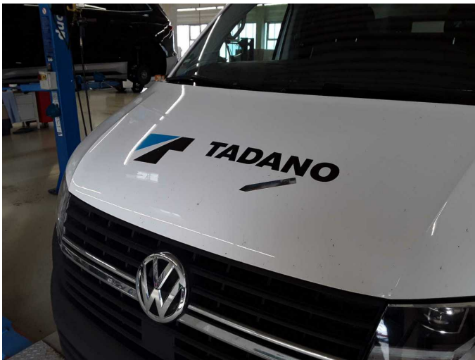
Damage 2: Bonnet: Bonnet - dent(s) - Smart repair
