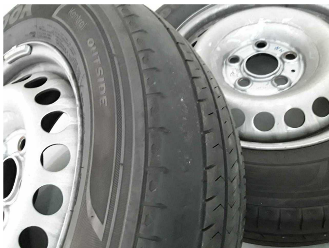
Damage 6: 2nd wheel set: 2 tyres - Worn - Replace
