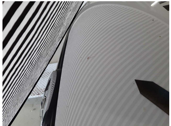
Damage 2: Bonnet: Bonnet - dent(s) - Smart repair
