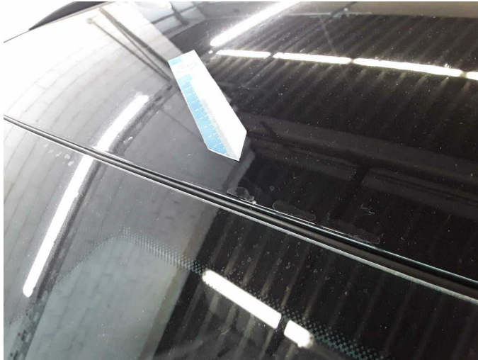
Wear and tear 4: Roof: Roof - Stone chips - No deduction
