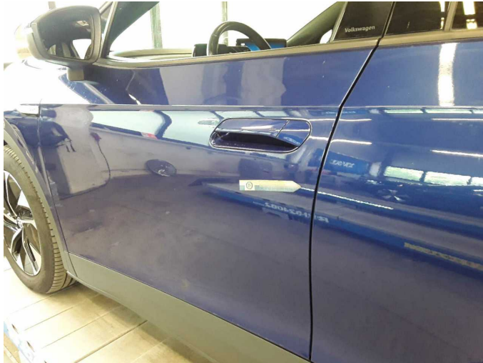
Damage 1: Door - front left side: Door - Scratch(es) - Smart repair
