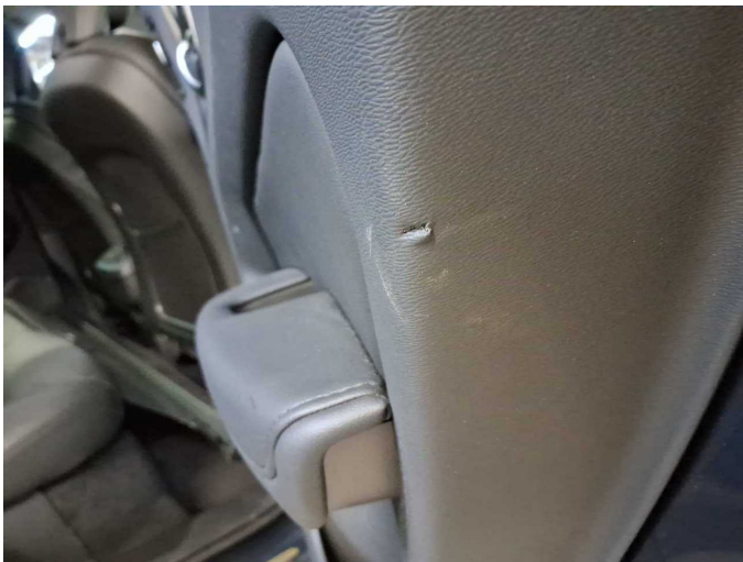
Damage 3: Trim / covers: Door trim - rear right side - Broken / torn - Smart repair
