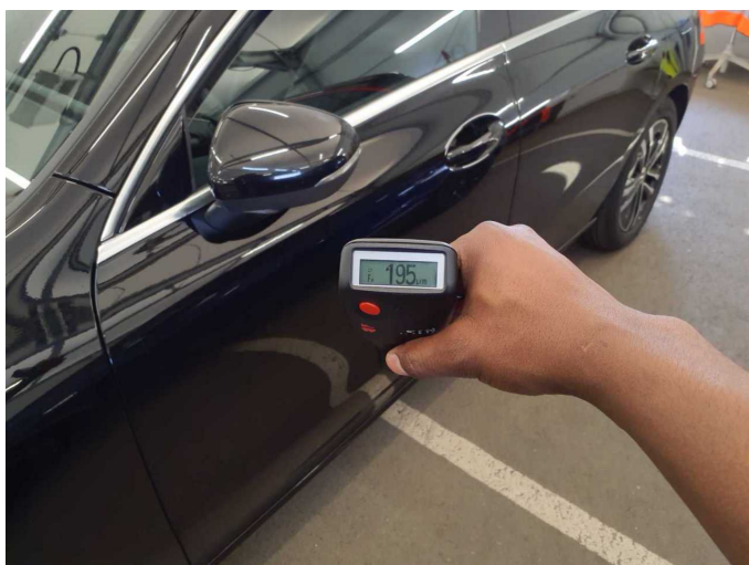
Repainting 3: Door - front left side
