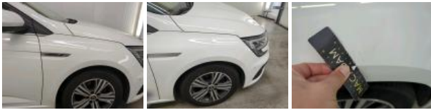
Outer door handle FR, Scratch(es), Repair and paint (complete)
