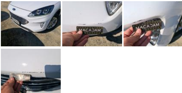
Bumper grille, Broken, Replace
