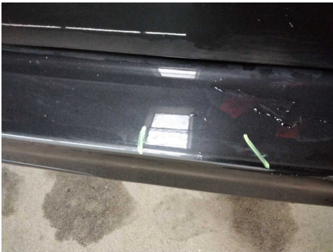
Damage 7: Rear bumper: Rear bumper - Scratch(es) - Paint
