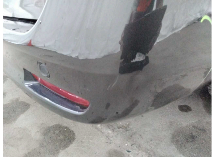
Damage 7: Rear bumper: Rear bumper - Scratch(es) - Paint
