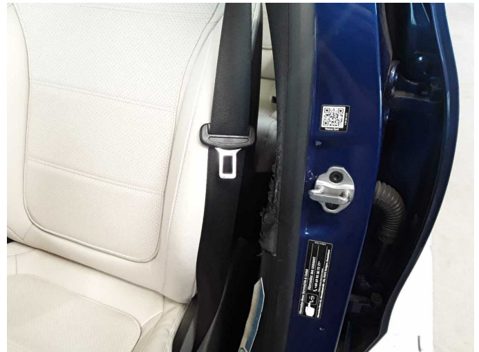
Damage 1: Trim / covers: B-pillar - trim - interior, left side - Damaged - Replace
