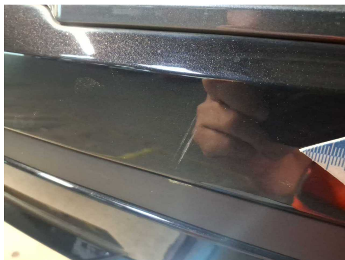
Damage 5: Rear bumper: Spoiler - Scratch(es) - Smart repair
