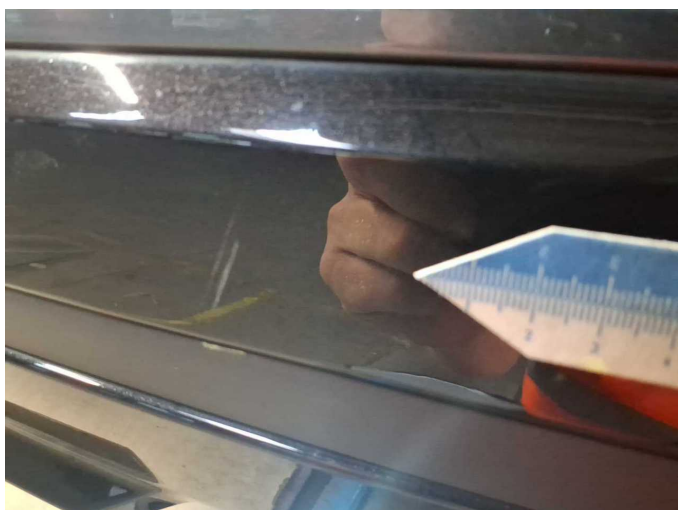
Damage 5: Rear bumper: Spoiler - Scratch(es) - Smart repair
