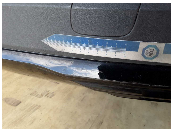
Damage 6: Rear bumper: Spoiler - Scratched - Replace
