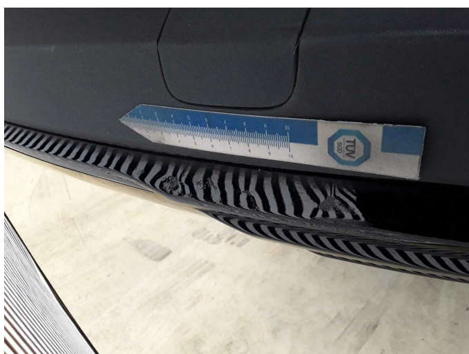
Damage 6: Rear bumper: Spoiler - Scratched - Replace
