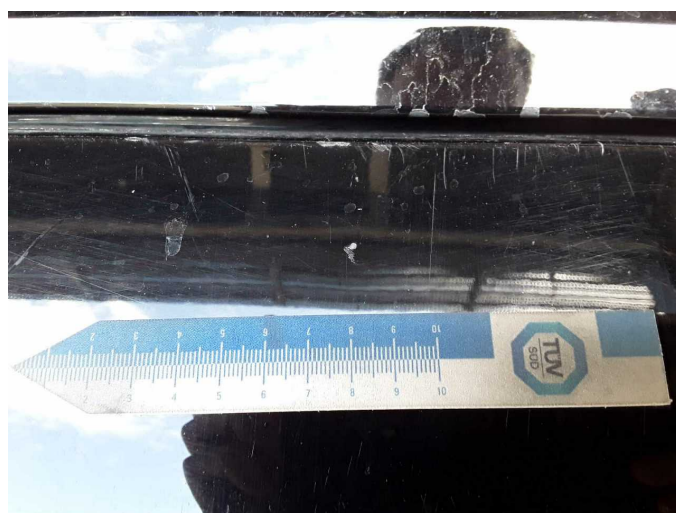
Damage 5: Rear bumper: Rear bumper - Scratch(es) - Paint
