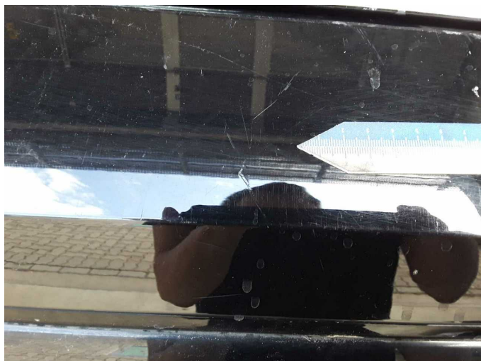
Damage 5: Rear bumper: Rear bumper - Scratch(es) - Paint
