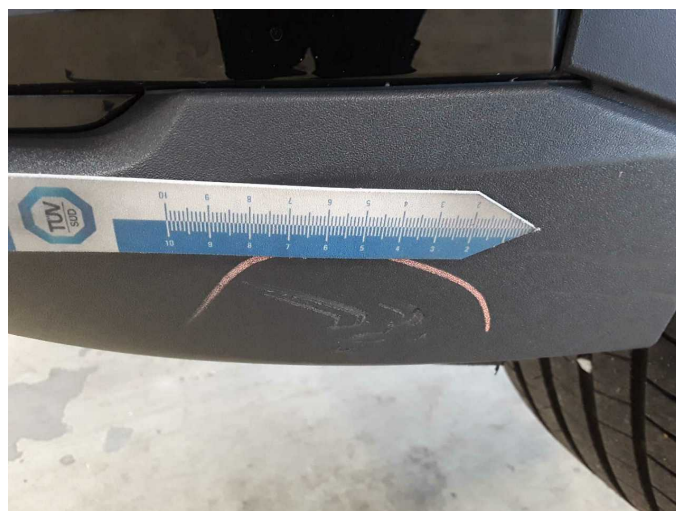
Damage 3: Front bumper: Spoiler (Links) - Scratch(es) - Replace
