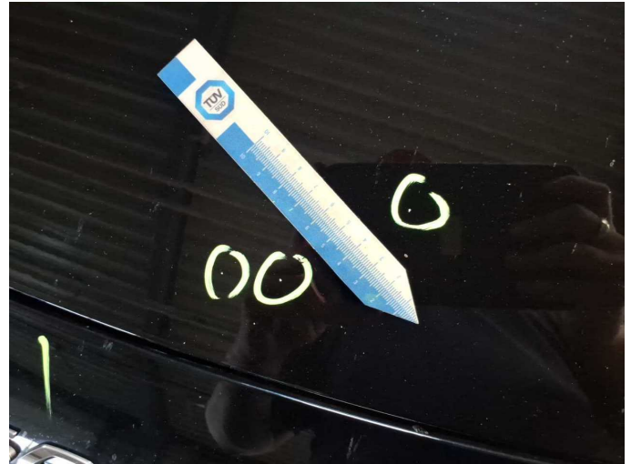
Damage 16: Bonnet: Bonnet - Stone chips - Paint
