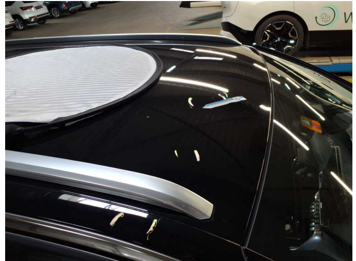
Damage 5: Roof: Roof - dent(s) - Smooth repair work
