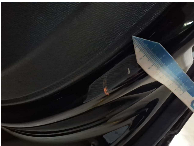
Damage 13: Door - rear right side: Door (Innenseite) - Dent / paintcoat damage - Repair and paint
