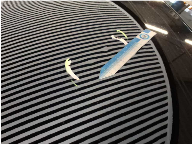
Damage 5: Roof: Roof - dent(s) - Smooth repair work
