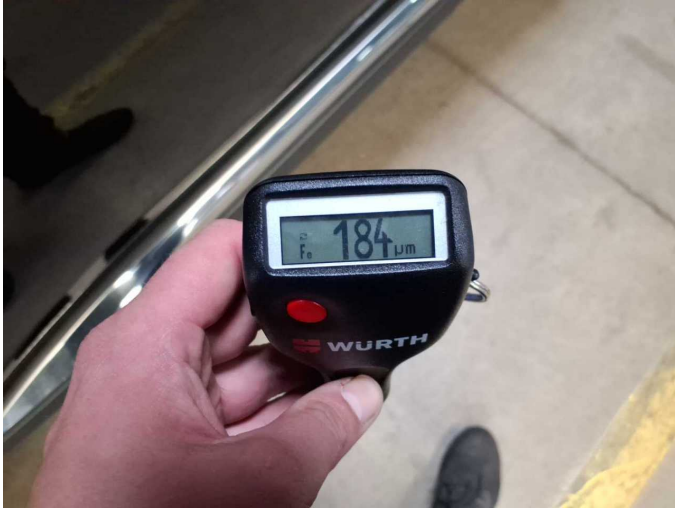
Repainting 1: Door - front left side
