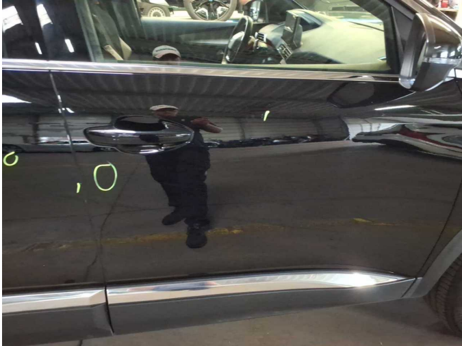
Damage 14: Door - front right side: Door - Dent / paintcoat damage - Repair and paint
