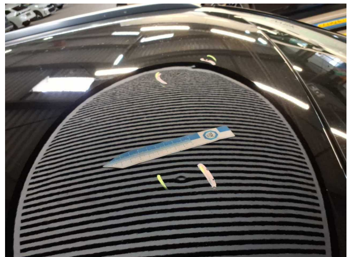
Damage 5: Roof: Roof - dent(s) - Smooth repair work
