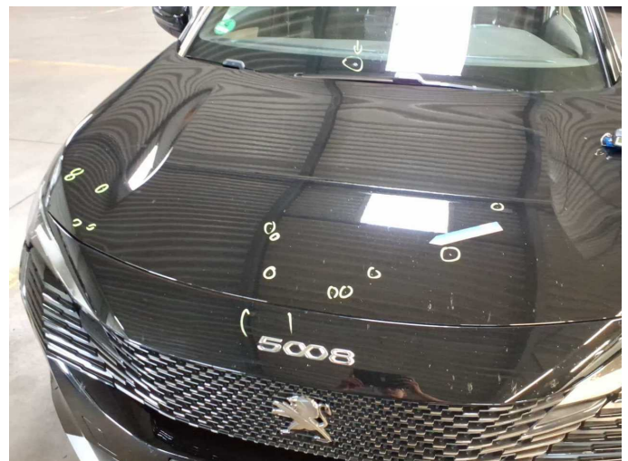
Damage 16: Bonnet: Bonnet - Stone chips - Paint
