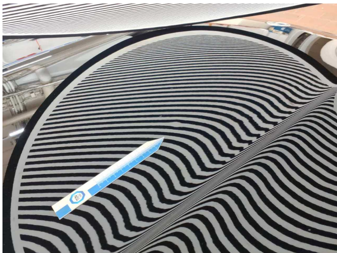
Damage 1: Bonnet: Bonnet - dent(s) - Smooth repair work
