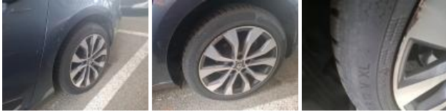
Tyre FR, Tear, Replace
