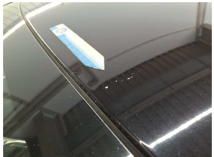
Damage 2: Roof: Roof - Stone chips - Paint
