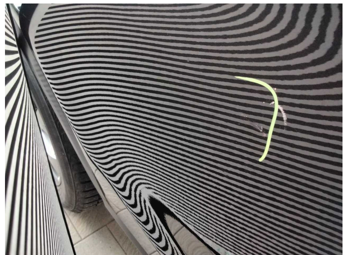
Damage 2: Door - rear right side: Door - Scratch(es) - Smart repair
