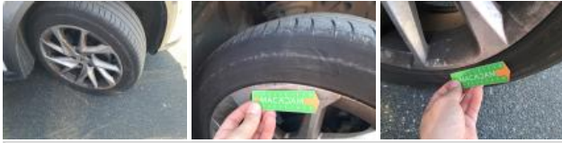
Tyre FR, Out of tolerance, Replace
