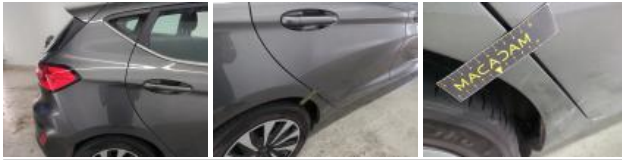
Door FR, Scratch(es), Repair and paint (complete)
