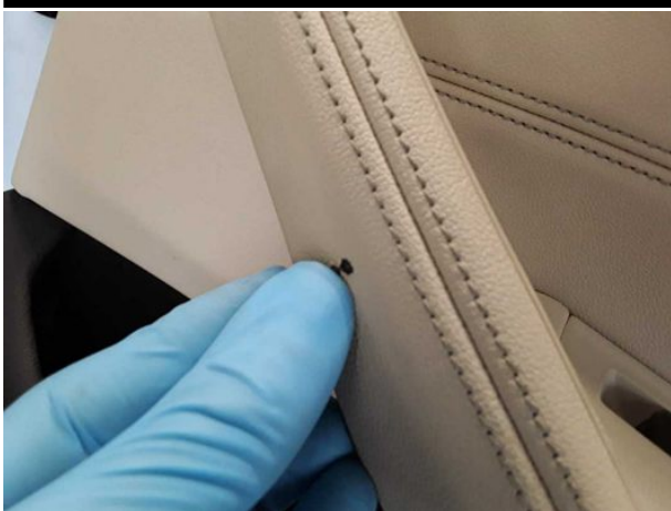
Damage #6: Trim / covers: Door trim - rear right side - Broken / to... - Loss in value
