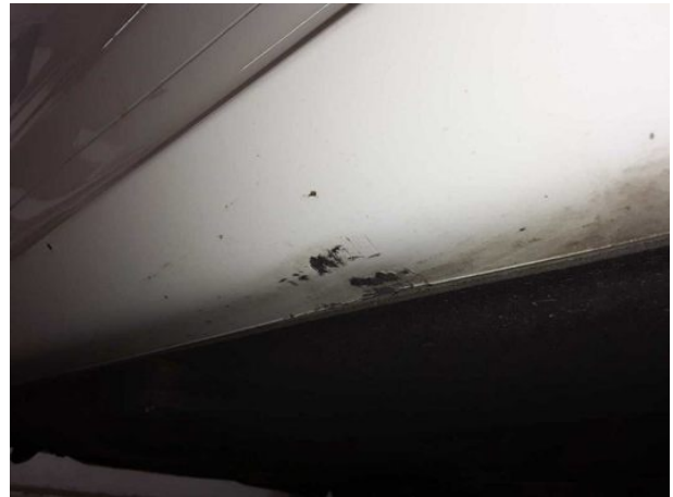
Damage #10: Sill - left side: Trim - Scratched - Repair and paint
