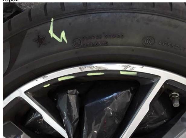
Damage #9: 2nd wheel set: 2 alloy rims - Scratched - Loss in value
