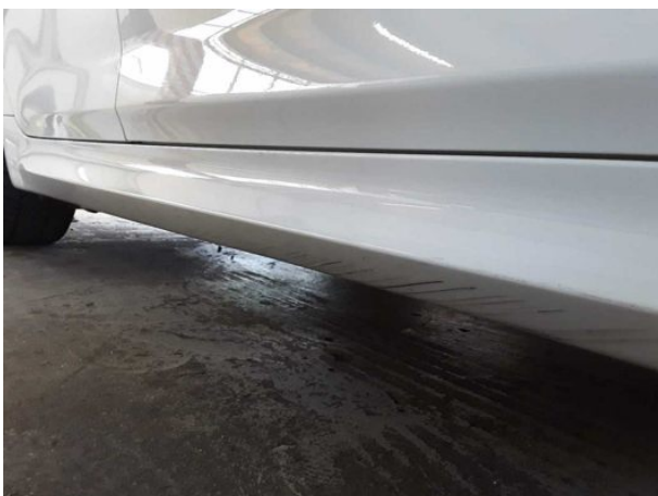
Damage #11: Sill - right side: Trim - Scratched - Repair and paint
