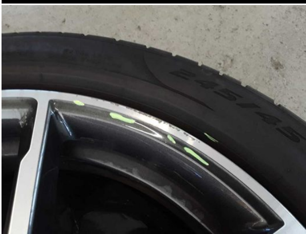
Damage #9: 2nd wheel set: 2 alloy rims - Scratched - Loss in value
