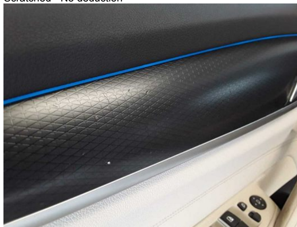
Damage #4: Trim / covers: Brightware / decorative strip (Tür) - Scratched - Loss in value
