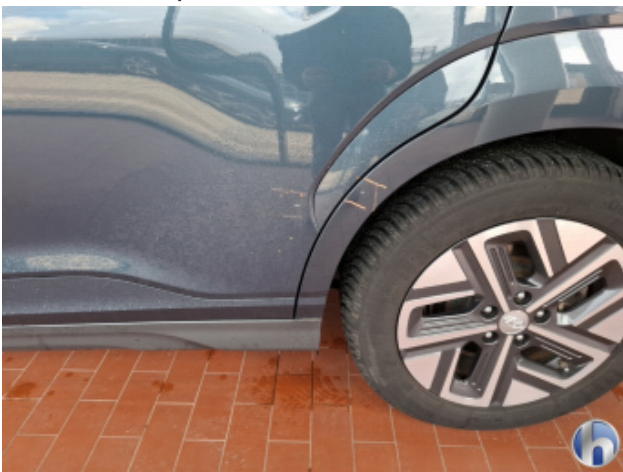
7. Tür Hinten - Links Kratzer - Smart Repair
