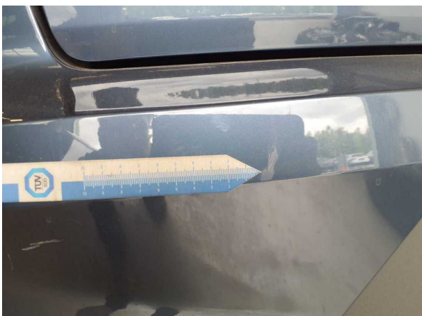
Damage #4: Rear bumper: Rear bumper - Scratch(es) - Paint
