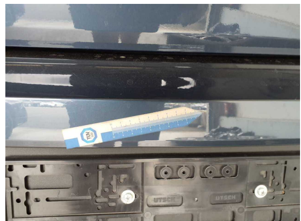
Damage #4: Rear bumper: Rear bumper - Scratch(es) - Paint
