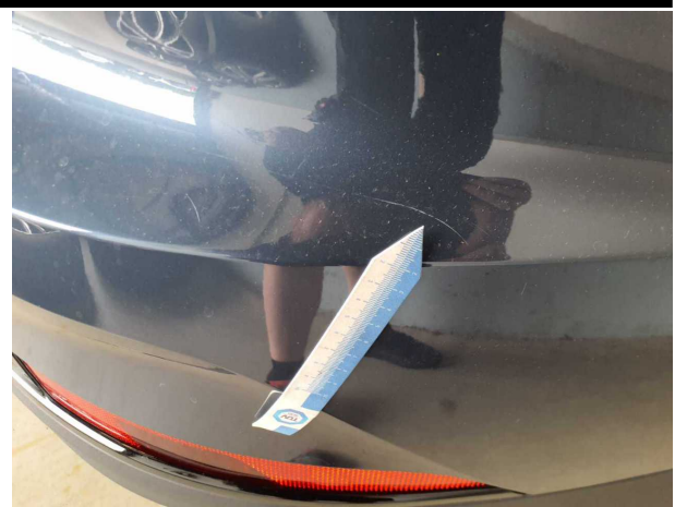
Damage #4: Rear bumper: Rear bumper - Scratch(es) - Paint
