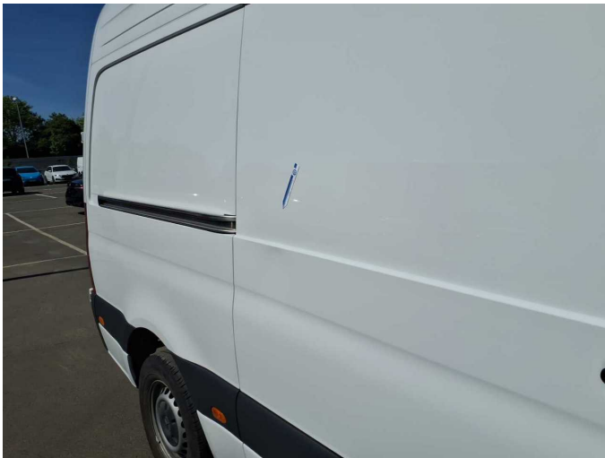
Damage 3: Sliding door, right: Sliding door - Deformed - Smart repair
