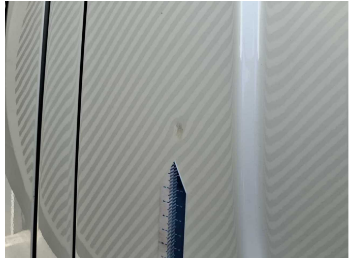
Damage 2: Side panel - rear left side: Side panel - Dent / paintcoat damage - Smart repair
