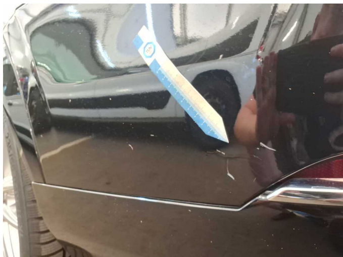
Damage 9: Rear bumper: Rear bumper - Scratch(es) - Paint
