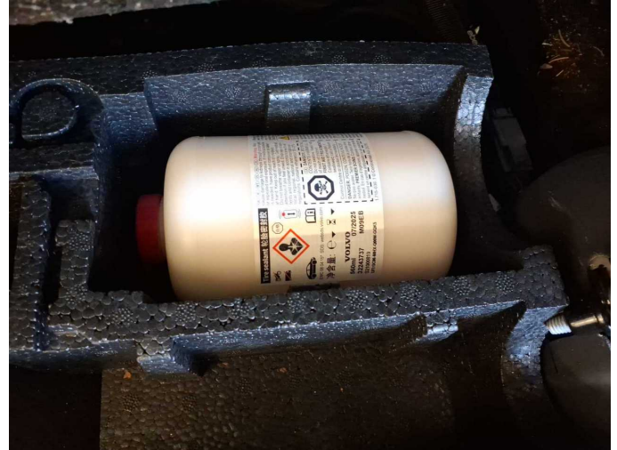
Damage 2: Equipment: Tirefit filler - Expired - Replace
