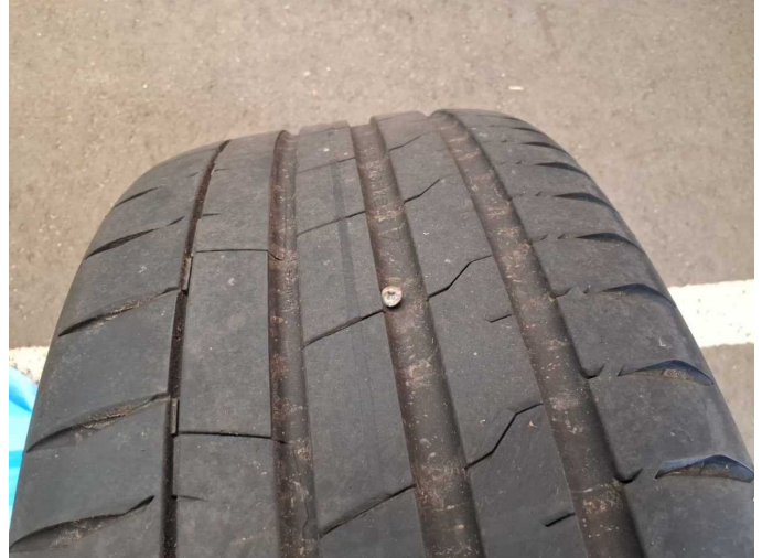
Damage 5: 2nd wheel set: 1 tyre (Nagel im Reifen) - Damaged - Replace
