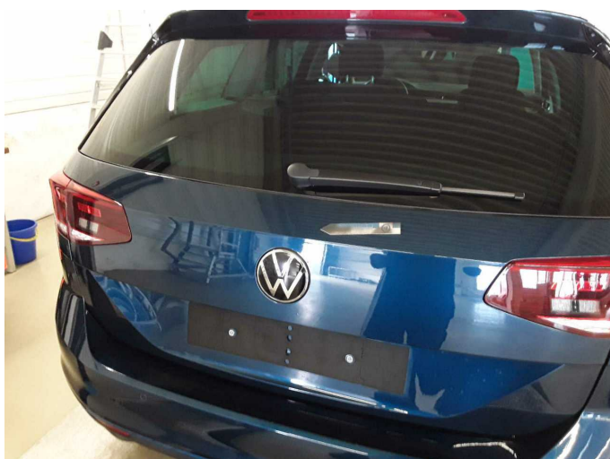
Damage 1: Boot lid / rear door: Boot lid glazed - dent(s) - Smart repair
