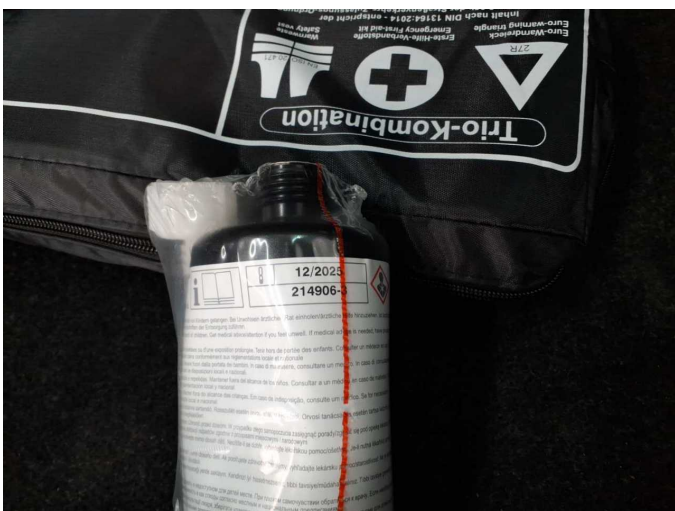
Damage 1: Equipment: Tirefit filler - Expired - Replace
