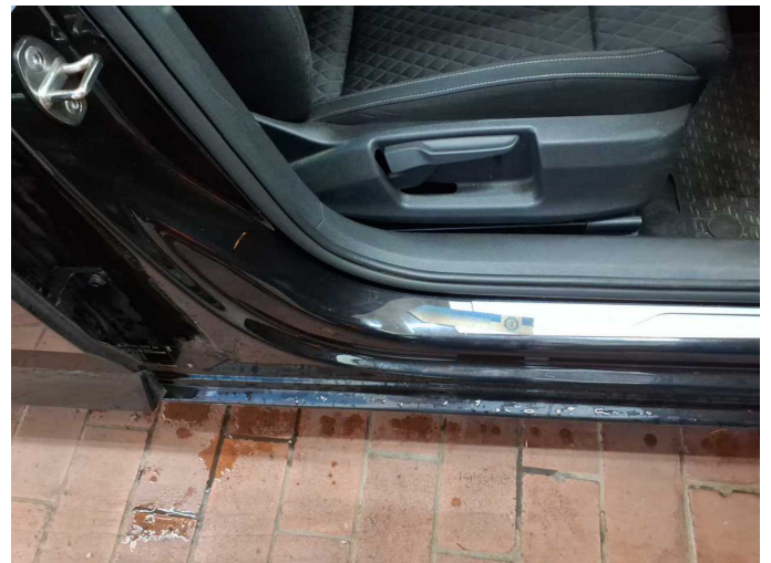
Damage 4: Sill - right side: Sill - dent(s) - Smart repair
