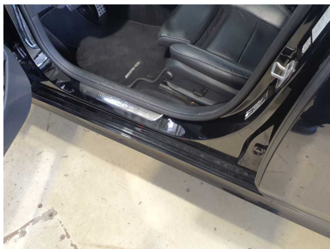
Damage 4: Sill - left side: Sill - Glued / labelled - Smart repair
