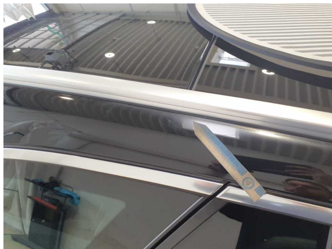
Damage 6: Roof: Roof rail - right side (Lack Nebel) - Paint defect - Conditioning
