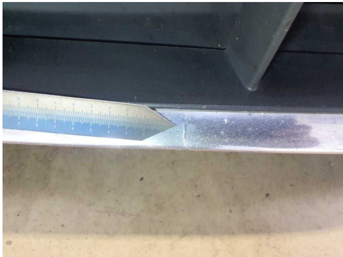
Damage 15: Trim / covers: Trim / covers - Scratch(es) - Replace
