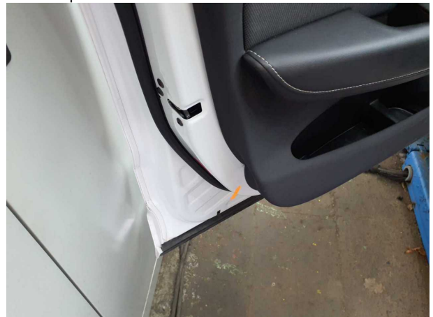
Beschädigung #14: Tür vorn links: Tür (innen) - Delle / Lackschaden - Smart Repair
