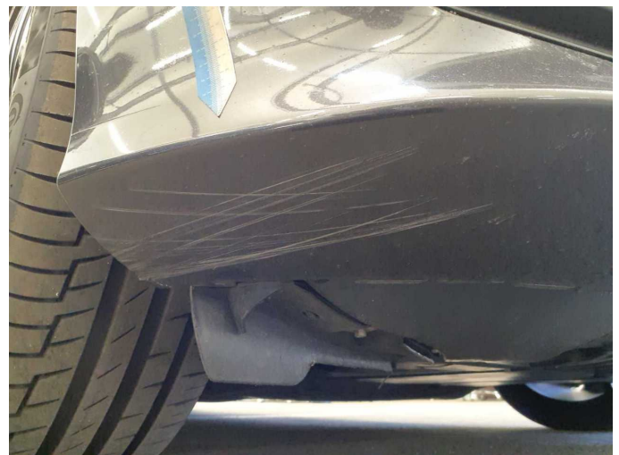
Damage 5: Front bumper: Front bumper - Scratch(es) - Paint
