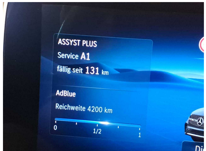
Damage 4: Misc.: Inspection / maintenance - Expired - Perform
