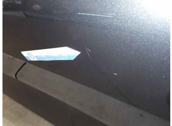
Damage 6: Door - front right side: Door - Scratch(es) - Paint
