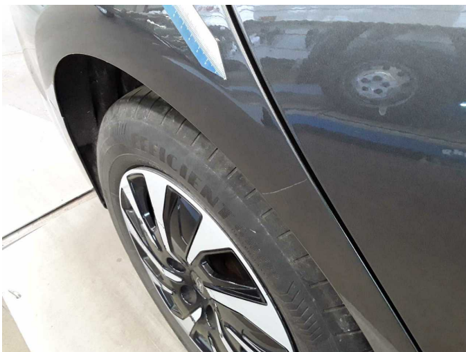
Damage 2: Side panel - rear right side: Side panel - Scratch(es) - Smart repair
