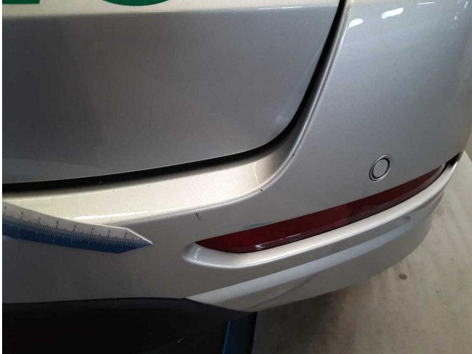
Damage 8: Rear bumper: Rear bumper - Scratch(es) - Paint
