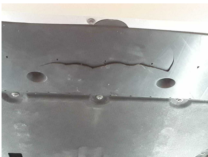
Damage 5: Body: Underbody panelling - Broken / torn - Replace
