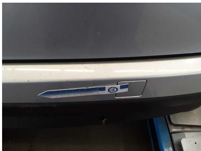
Damage 8: Rear bumper: Rear bumper - Scratch(es) - Paint
