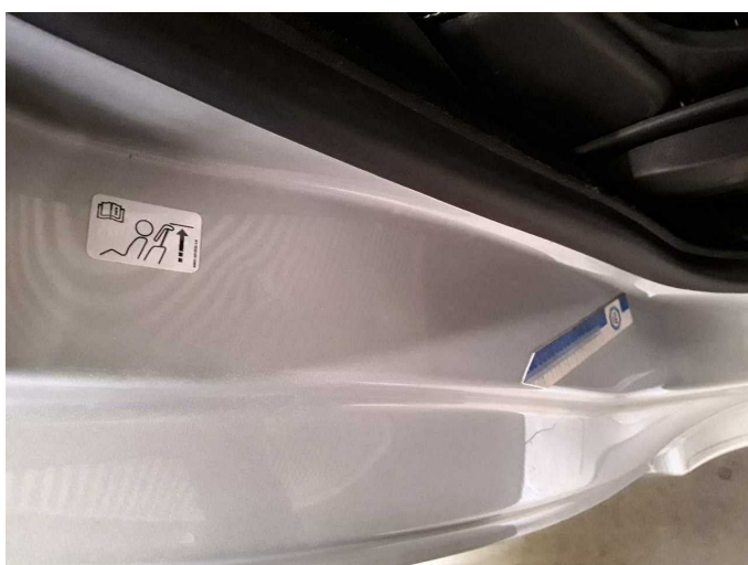
Damage 4: Side panel - rear right side: Sill - Dent / paintcoat damage - Smart repair
