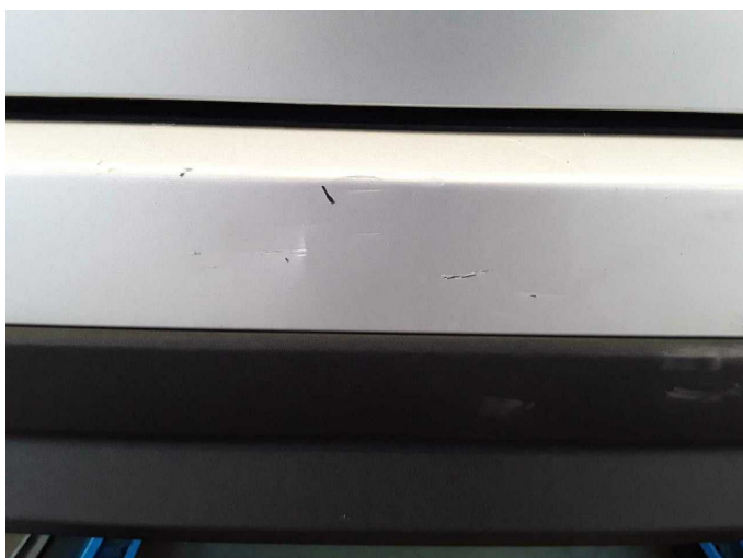
Damage 8: Rear bumper: Rear bumper - Scratch(es) - Paint
