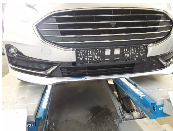
Damage 6: Front bumper: Front bumper - Dent / paintcoat damage - Repair and paint
