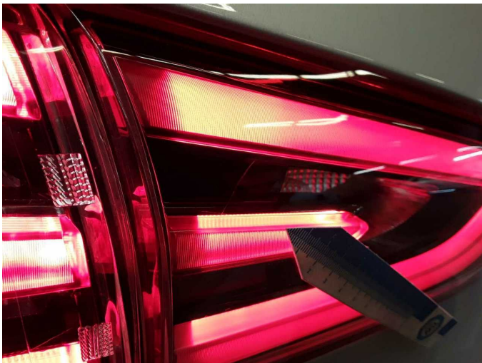
Wear and tear 1: Tail light: Auxiliary brake light - Scratch(es) - No deduction
