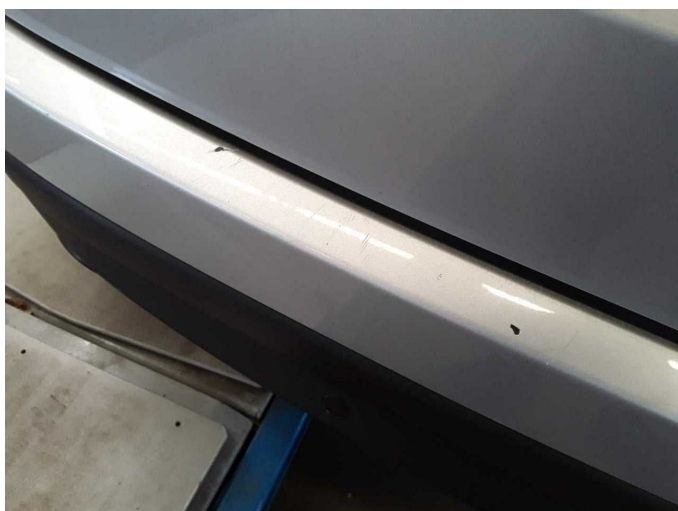
Damage 8: Rear bumper: Rear bumper - Scratch(es) - Paint
