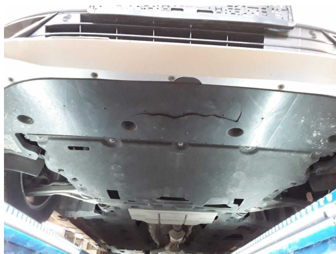
Damage 5: Body: Underbody panelling - Broken / torn - Replace
