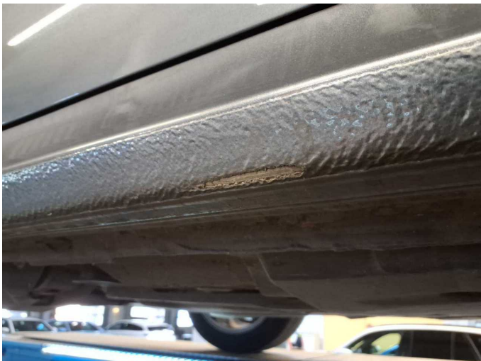
Damage 1: Sill - right side: Sill - Paint defect - Smart repair
