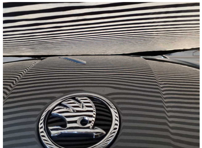
Damage 4: Bonnet: Bonnet (Verformt) - Dent / paintcoat damage - Repair and paint
