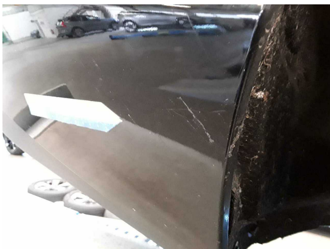
Damage 6: Rear bumper: Rear bumper - Scratch(es) - Paint
