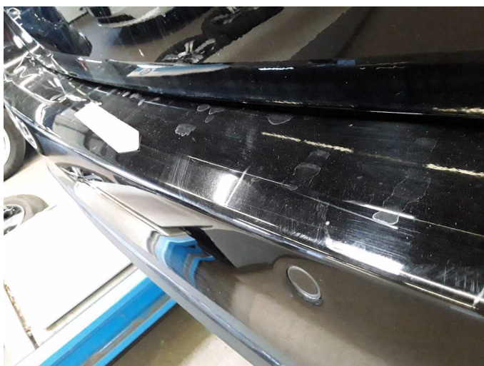
Damage 6: Rear bumper: Rear bumper - Scratch(es) - Paint
