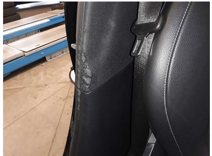
Damage 3: Trim / covers: B-pillar - trim - interior, right side - Damaged - Replace
