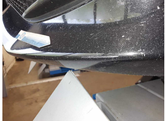
Damage 4: Front bumper: Front bumper - Scratched - Paint
