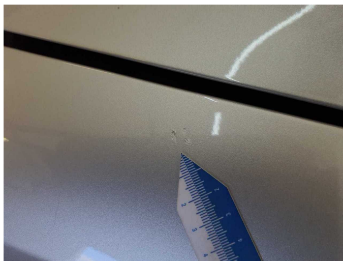
Damage 4: Mudguard - left side: Mudguard - left side - Stone chips - Smart repair
