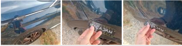
Door FL, Dent(s) and scratch(es), Acceptable
