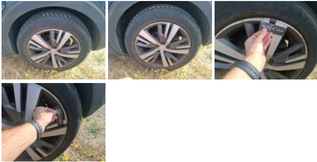
Tyre RL, Out of tolerance, Replace
