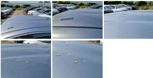
Roof, Hail damage, Repair and paint (complete)
