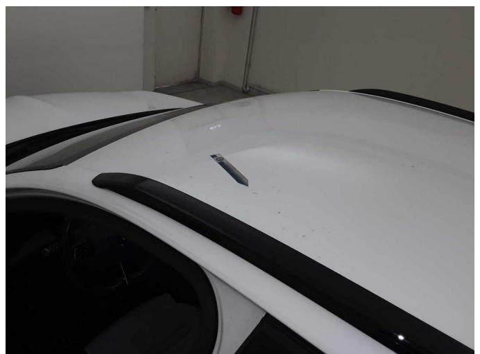
Damage 4: Roof: Roof (Baumharz) - Soiled - Clean
