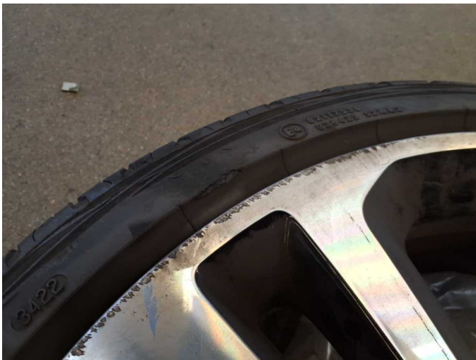
Damage 7: 2nd wheel set: 1 tyre - Damaged - Replace
