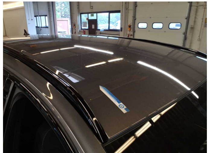
Damage 4: Roof: Roof - dent(s) - Smooth repair work
