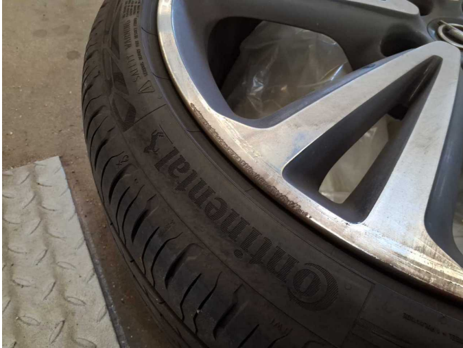
Damage 9: 2nd wheel set: 2 alloy rims - Scratched - repair according to calculation
