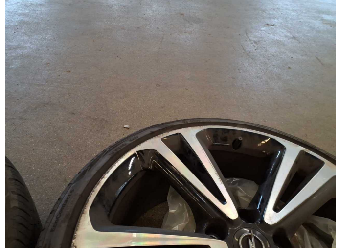
Damage 7: 2nd wheel set: 1 tyre - Damaged - Replace
